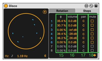
The Steps tab allows you to go further with experimentation by individually changing the position/phase (15), volume (16), pan (17), and mute control (18) for every single step.
