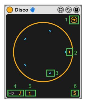
All the delay lines are distributed in a time range defined by (5), both in sync and free hz mode (4).
